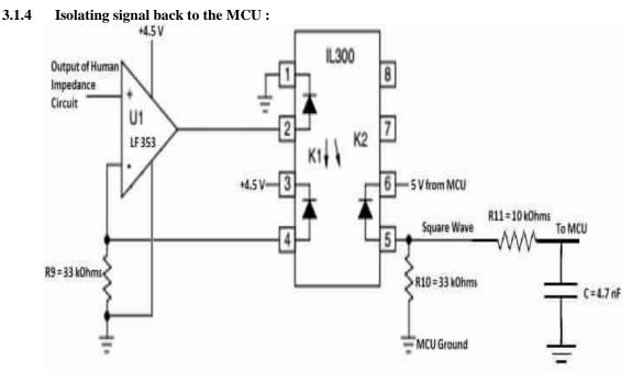
The isolating circuit is the same as the one used in previous case. So we are using power rails of the microcontroller unit to provide a stable signal for the ATMEGA1284. Resistors R9 and R10 are equal to each other to ensure unity gain since we want the output equal to the input. We need a low pass filter which was used to smooth out the signal so the microcontroller can perform calculations on the data from the signal.
